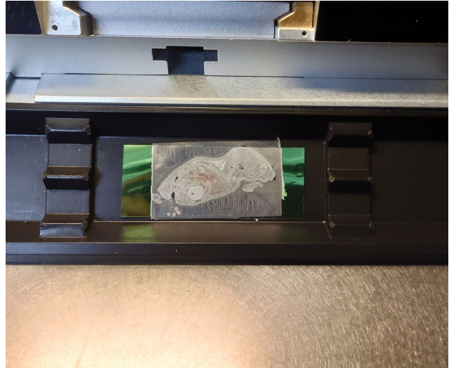
An adhesive film: LMD film type 2(13S2) The thickness of the section: 8 micron
